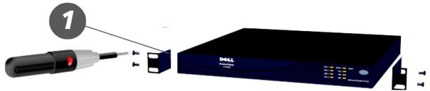
It is important that you use the black screws, and make sure that the mounting brackets are securely connected to the unit. These brackets will hold the entire weight of the unit.
